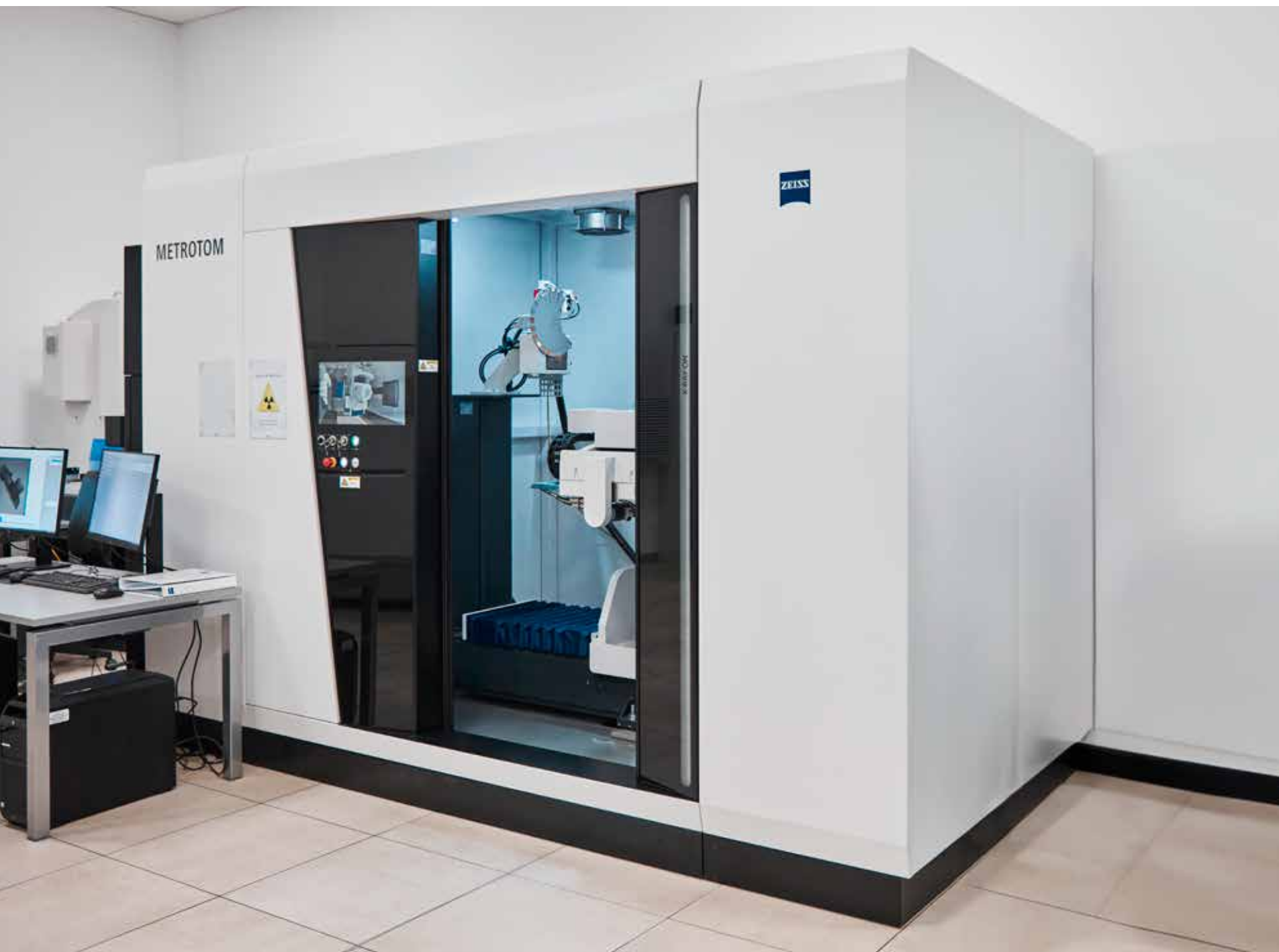
The new CT ZEISS Metrotom 1500 machine.
